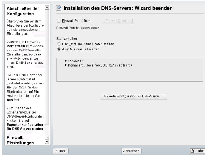
Abbildung 22.3 DNS-Server-Installation: Assistent beenden
