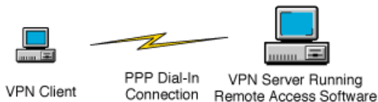
Figure 19 VPN Client Using a Direct Dial-In Connection
