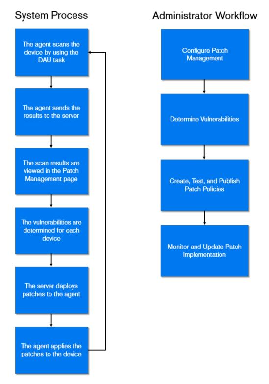
The patch detection (PD) cycle begins each day at the ZENworks Server where a Vulnerability Detection task is scheduled for all ZENworks managed devices (servers and workstations).
