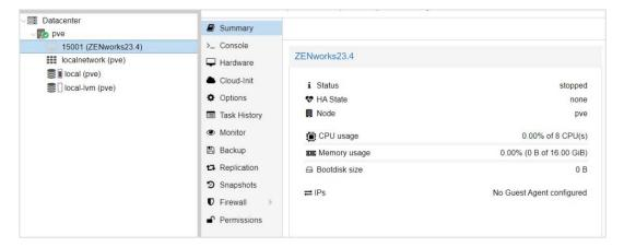
b. Click Hardware. This displays the list of hardware. The disk that you created using the .vmdk file is also displayed in the hardware list as Unused Disk 0 along with the storage name appended in the description. This Unused Disk 0 is the first hard disk of the appliance, which is created under the local-lvm storage.
