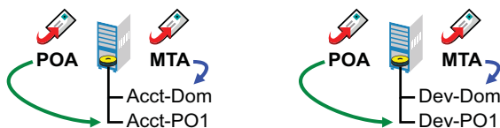
Figure 8-6 Agent Software on the Same Server with the Domain and Post Office
