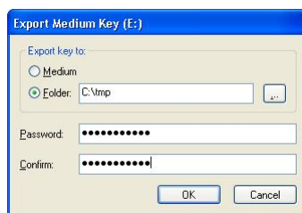
Figure 156: Export Medium Key dialog - to export the encryption key to a file
